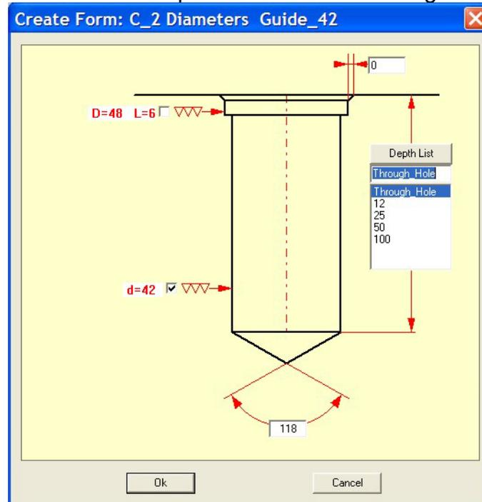
Since this will be a through hole for the Guide pins, we need we need to check the box **d=42**
