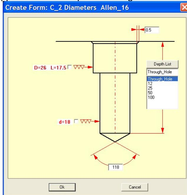
Change the settings as shown above. Disable the reaming of this drill form for the cylinders. Click on . Click on the **8 red points** (Mastercam color 12). Click on **Enter**. The following will be the result.
