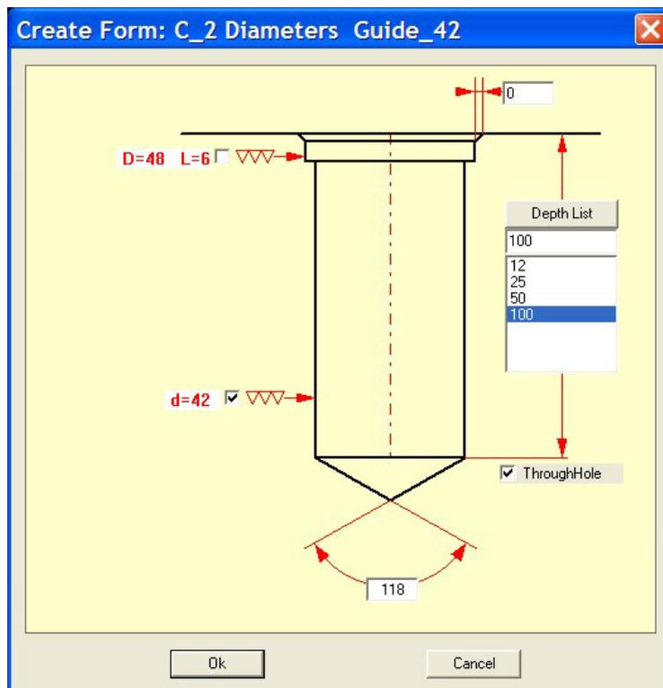
Set the parameters as shown above. Notice that the 42mm diameter is checked **d=42**  – indicating that it should be reamed. Click on
