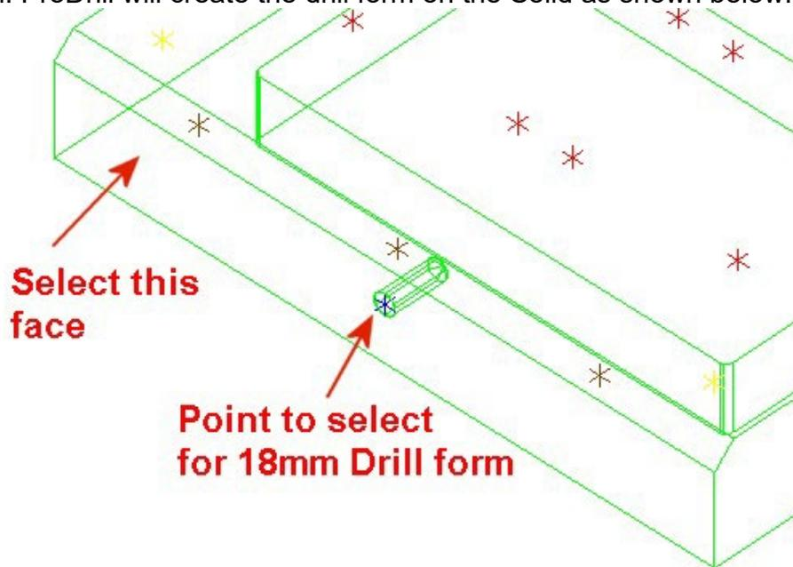
Notice that the form created has a 0.5mm chamfer at the start of the drill form and has a 118 drill tip form.
