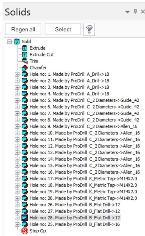
You can now process all the Drill Forms using ProDrill. Click on **Forms View** icon to process the part. All the Forms are recognized. When you apply drilling processes to them, the following is the result:
