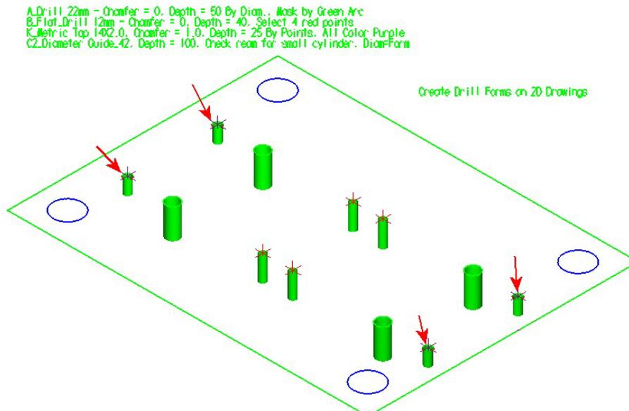
To indicate a Tap form, ProDrill also creates a 270 degree red arc on top of the cylinder to be tapped. Notice that the arc is created below the chamfer. The image on the right shows that the tap form ends in a tooltip (angle used in the Forms Parameters).
