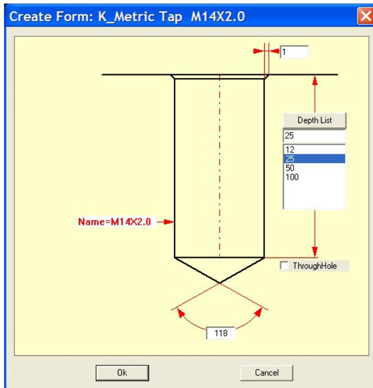
Set the parameters as shown above. Notice that we are creating a 1mm chamfer and creating it as a blind hole (**ThroughHole** unchecked). Click on
